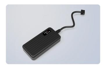
V series asset tracker is an intelligent vehicle monitoring terminal. The device integrates CAT.1/CAT.M/GSM/NBIOT, GNSS, Wi-Fi, Bluetooth, a variety of sensors and extended GPIOs. It contains several variants covering different regions and networks around the world.
